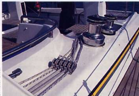
Above, all the major control lines are led back to the cockpit through a bank of Antal clutches (right) to Andersen winches. Far right, reaching in 20 knots of true wind
